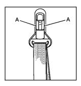
To move it up or down, squeeze the release buttons (A) together and move the height adjuster to the desired position.
